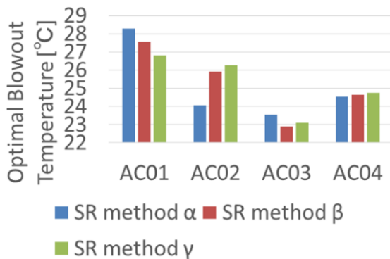
Fig.4 Optimal blowout temperature from SR method
