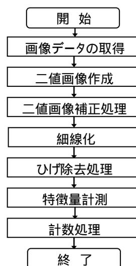
Fig.1 The flow chart for image processing of the AFACS .
