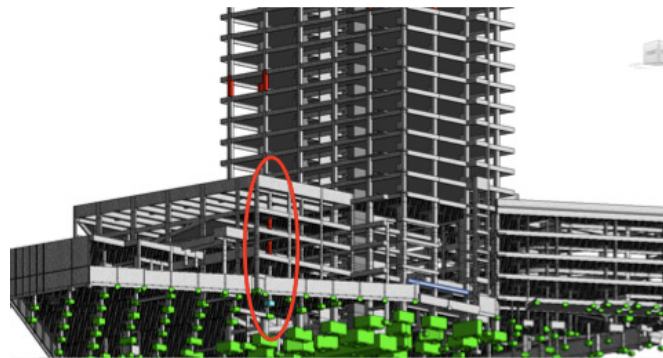
Figure 2. Line of non-conform columns above a non-conform foundation
