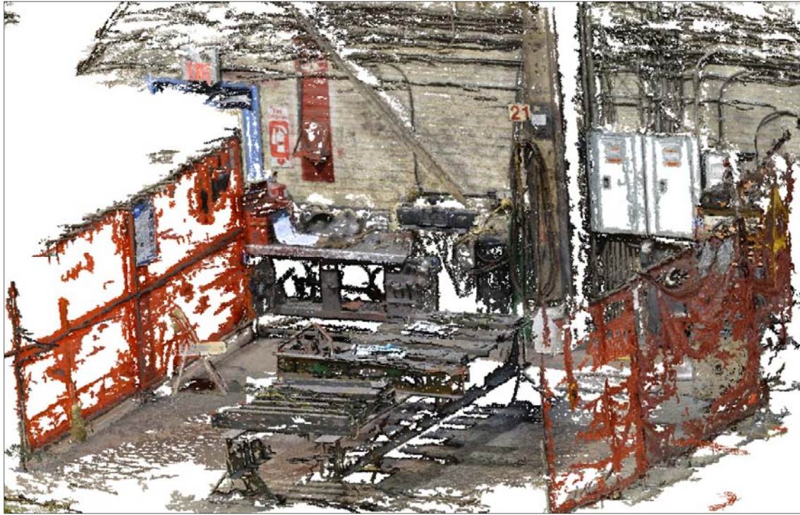
Figure 4. Point cloud data of the steel welding workplace
