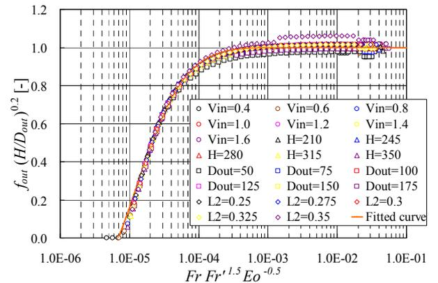
Fig. 12 Non-dimensional correlation for outflow fraction
