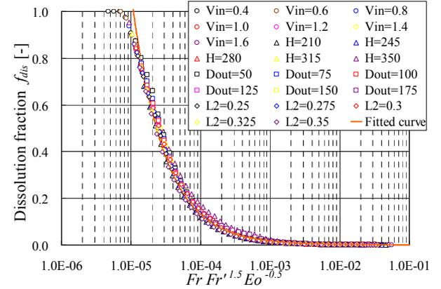
Fig. 11 Non-dimensional correlation for dissolution fraction
