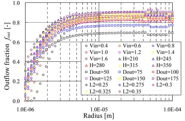
Fig. 10 Outflow fraction in parametric study
