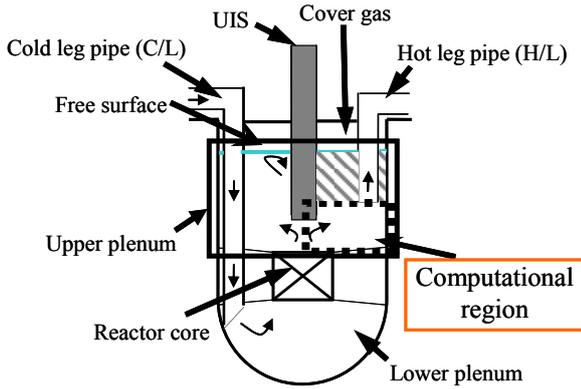
Fig. 1 Cross section of reactor vessel
