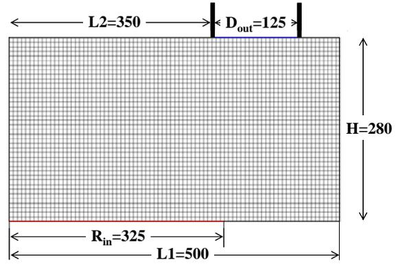
Fig. 3 Computational geometry and mesh arrangement (Reference case)
