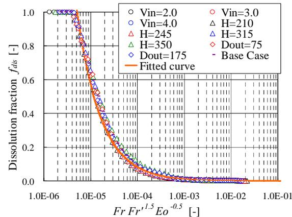
Fig.6 Non-dimensional correlation for dissolution fraction
