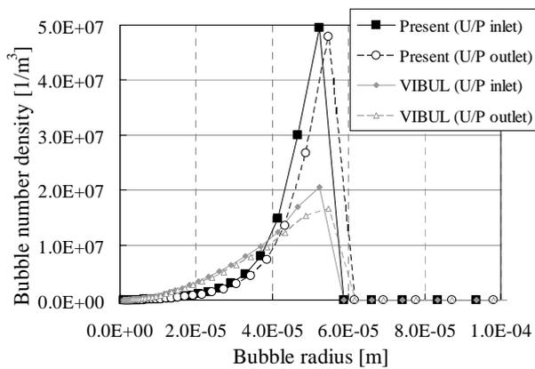
Fig. 12 Number density of gas bubbles with present dissolution model
