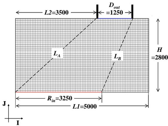
Fig.3 Computational geometry and mesh arrangement
