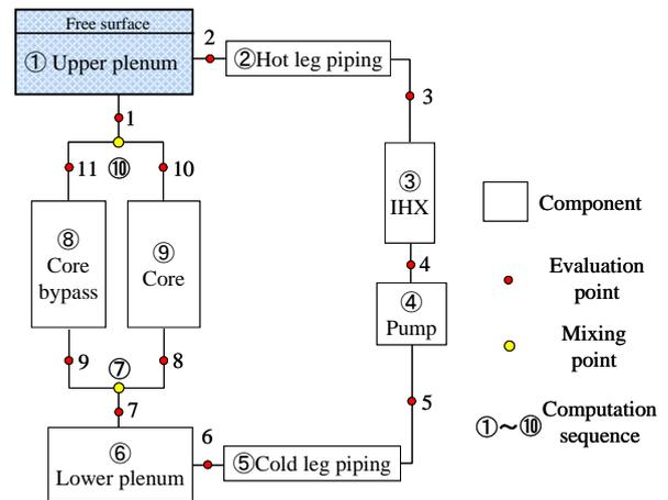
Fig.9 Nodalization of coolant system in VIBUL code
