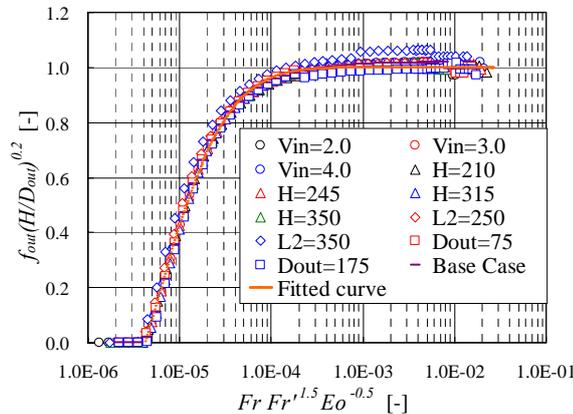
Fig.7 Non-dimensional correlation for outflow fraction
