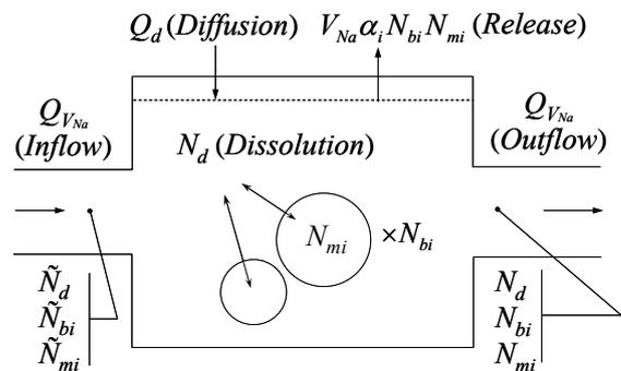
Fig.1 Conservation of gas bubbles in a plenum
