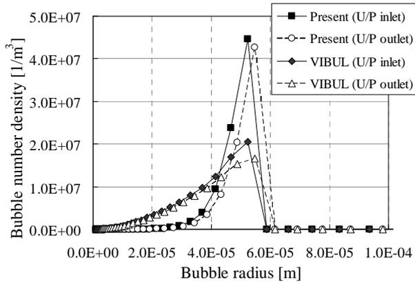
Fig. 10 Number density of gas bubbles with present model and VIBUL model
