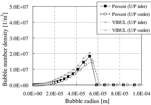
Fig. 11 Number density of gas bubbles with present release model
