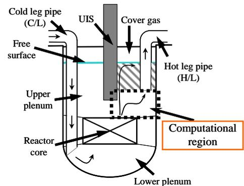
Fig.2 Cross section of reactor vessel
