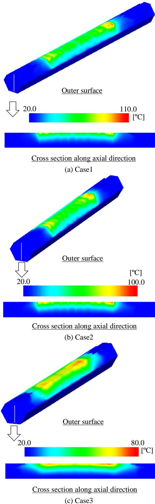
Fig. 8 Temperature distribution on outer surface and cross section along axial direction
