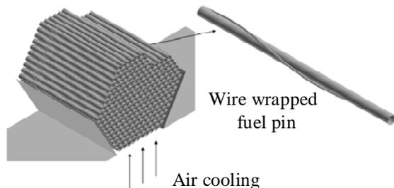
Fig. 1 Schematic of TRU fuel bundle and its cooling
