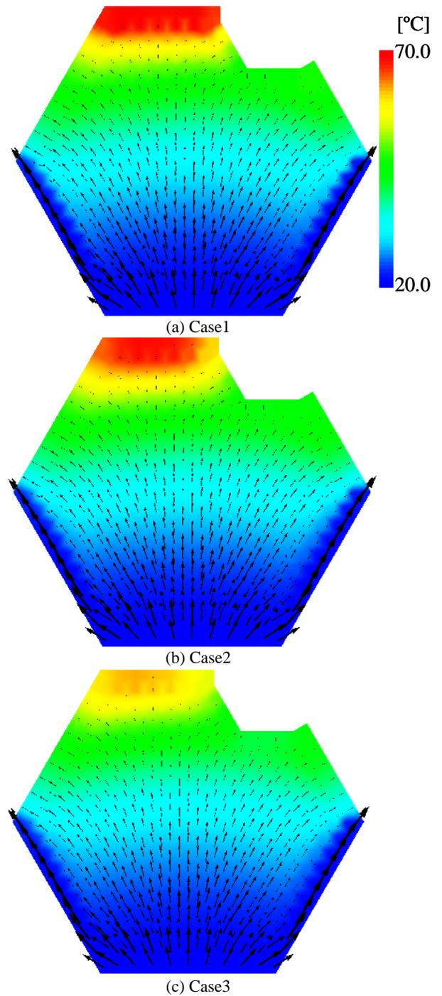
Fig.9 Velocity and temperature distribution at the center
