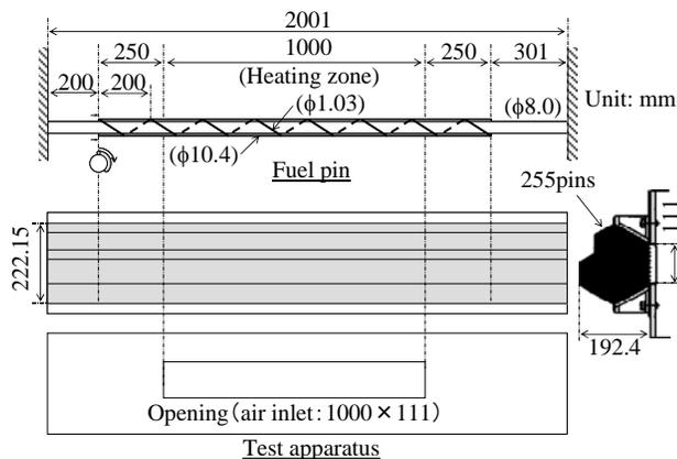
Fig. 7 Analytical geometry of mocked up test<sup>1</sup>
