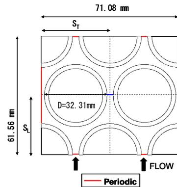
**Fig. 2 A staggered tube bank ( $P/D=1.1$ ).**
