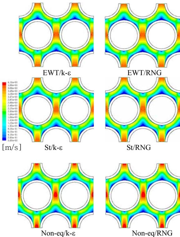
**Fig. 6** The distribution of magnitude of the velocity.
