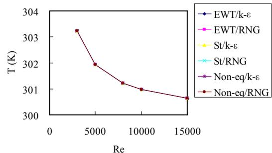
**Fig. 4 The average temperature of fluid  $T_m$  ( $P/D=1.2$ ).**
