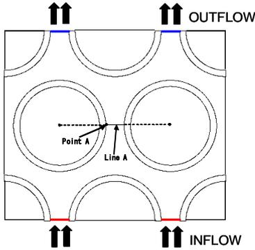
Fig. 3 Integral region and minimum gap.
