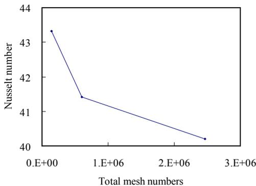
Fig. 10 The total number of dependence for Nusselt number when  $Re=3,000$  calculated in EWT and standard  $k-\epsilon$  model.
