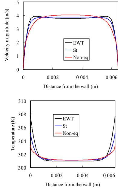
**Fig. 8** The magnitude of the velocity and temperature along the Line A (See Fig. 3).
