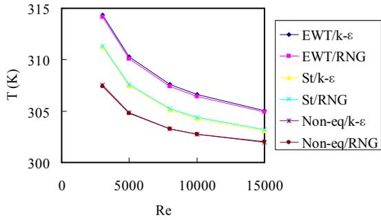
**Fig. 5** The temperature of tube surface  $T_w$  ( $P/D=1.2$ ).
