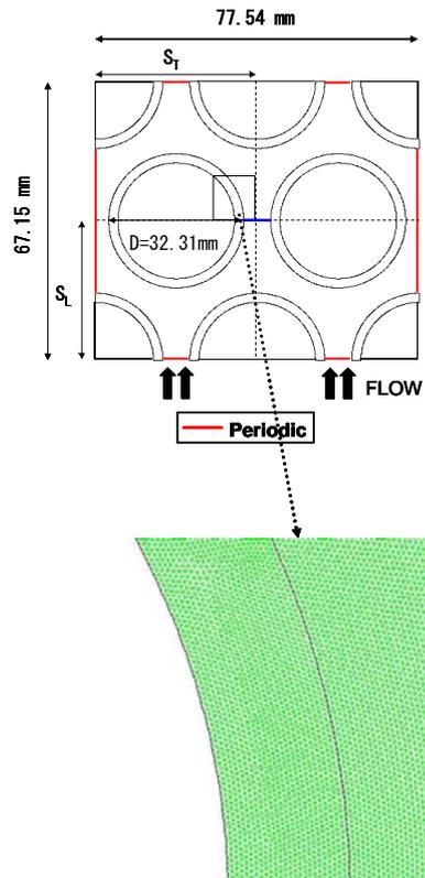
**Fig. 1 A staggered tube bank and mesh ( $P/D=1.2$ ).**
