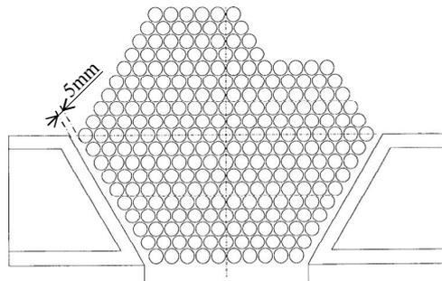
Fig. 5 Cross sectional view of bundle
