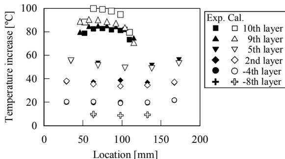
**Fig. 9 Comparison of cladding surface temperature increase (default)**
