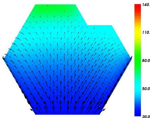
Fig. 14 Velocity and temperature distribution of coolant at the center (1.1mm clearance)
