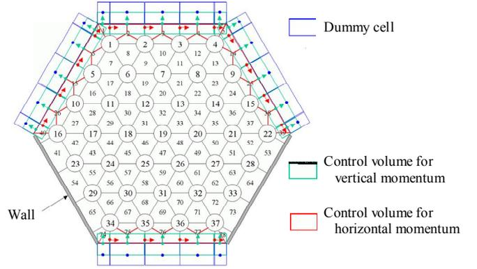
Fig. 3 Additional control volume for boundary condition
