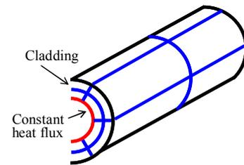
Fig. 6 Nodalization of fuel cladding
