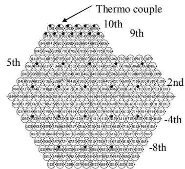
**Fig. 10 Location of temperature measurement (cladding surface)**
