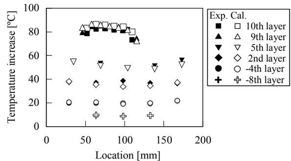
**Fig. 11 Comparison of cladding surface temperature increase (considering natural convection heat transfer at outermost fuel pins)**
