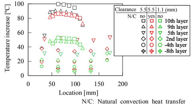
Fig. 15 Influence of clearance (cladding surface temperature)
