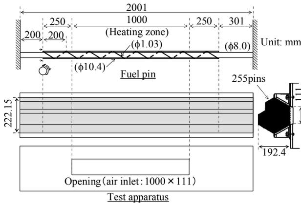
Fig. 4 Geometry of test apparatus
