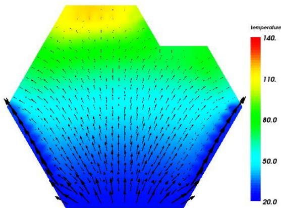
**Fig. 8 Velocity and temperature distribution of coolant at the center of heating zone**
