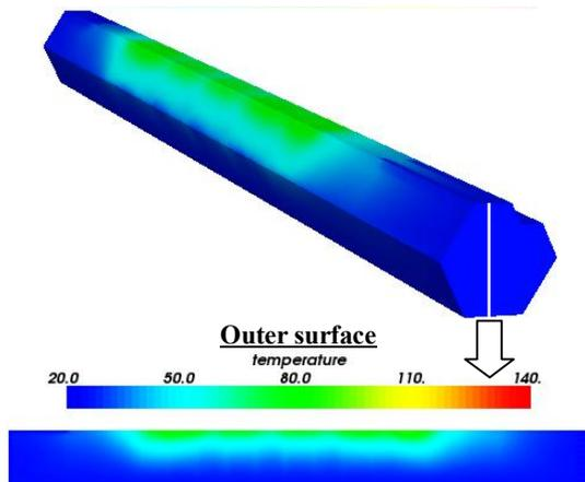
Fig. 13 Temperature distribution of coolant (1.1mm clearance)
