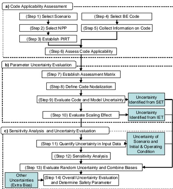
Fig. 3 SPLC quantification process with BE code.
