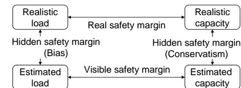
Fig. 1 Realistic and estimated load and capacity.
