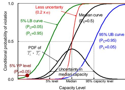
Fig. 8 Comparison of SPLC estimated and safety criterion.
