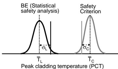
Fig. 7 Concept of load-capacity model.
