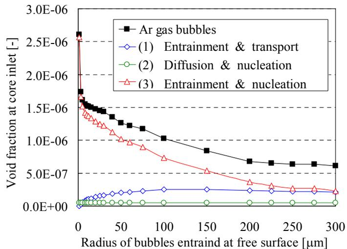
**Fig. 14 Void fraction at the core inlet as a function of the entrained bubble radius.**
