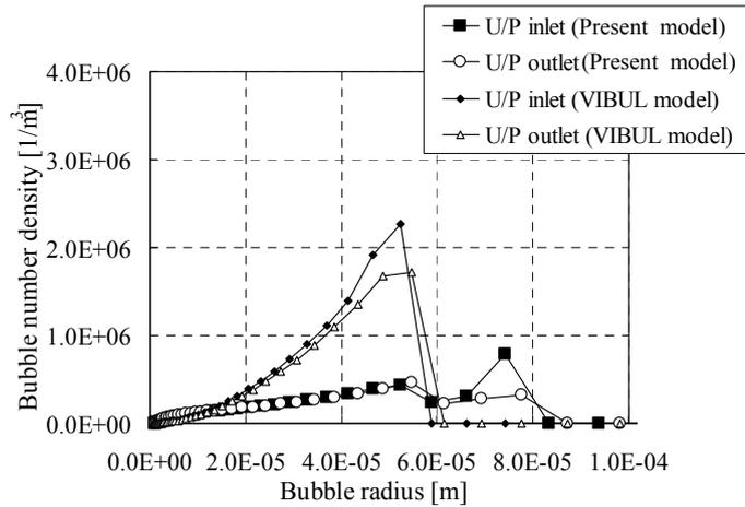
**Fig. 10 Gas bubble number density (argon and helium) in the upper plenum.**
