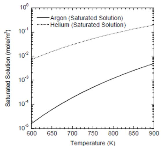
**Fig. 1 Solubilities of argon and helium in sodium for the SFR operating temperature.**
