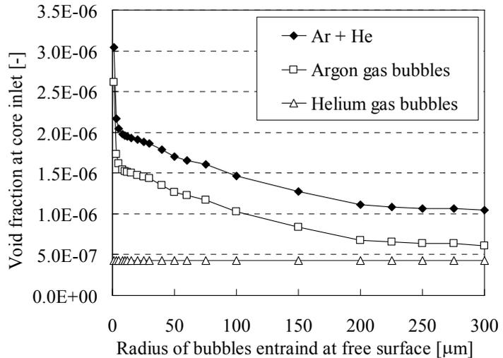
**Fig. 13 Void fraction at the core inlet as a function of the entrained bubble radius.**
