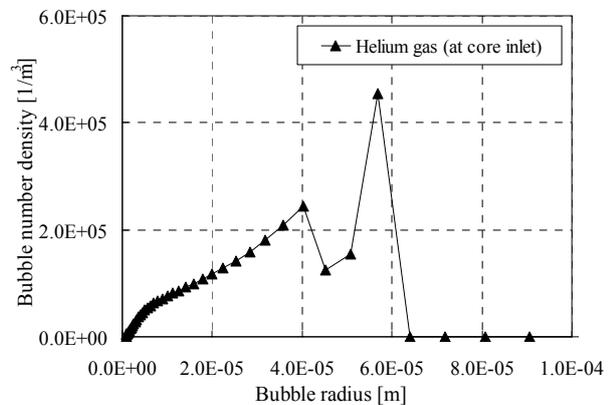
**Fig. 11 Helium bubble number density at the core inlet as a function of radius.**
