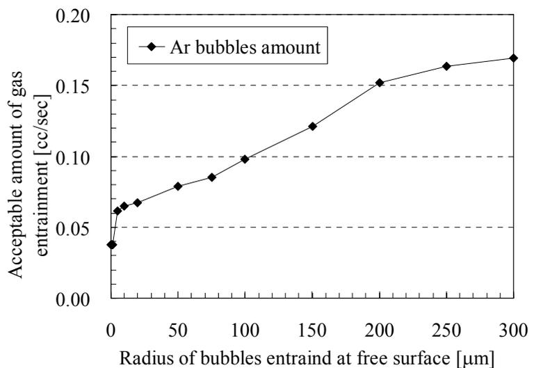
**Fig. 17 Design map in terms of the entrainment rate and the entrained bubble radius**
