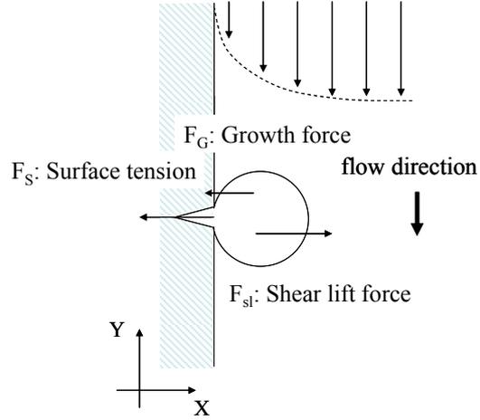
**Fig. 6 Force balance in flow direction. Fig. 7 Force balance in crossflow direction.**
