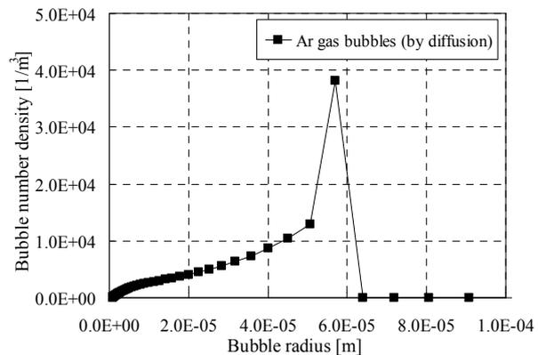
**Fig. 12 Bubble number density at the core inlet for the argon gas with no gas entrainment.**
