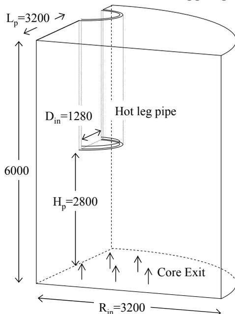
**Fig. 2 Computational domain of reactor upper plenum**
