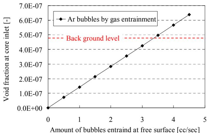
**Fig. 16 Void fraction at the core inlet as a function of the entrained bubble radius (entrained bubble radius is  $300 \mu\text{m}$ ).**
