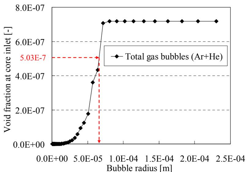
**Fig. 18 Relationship of removed bubble radius and void fraction at core inlet.**
