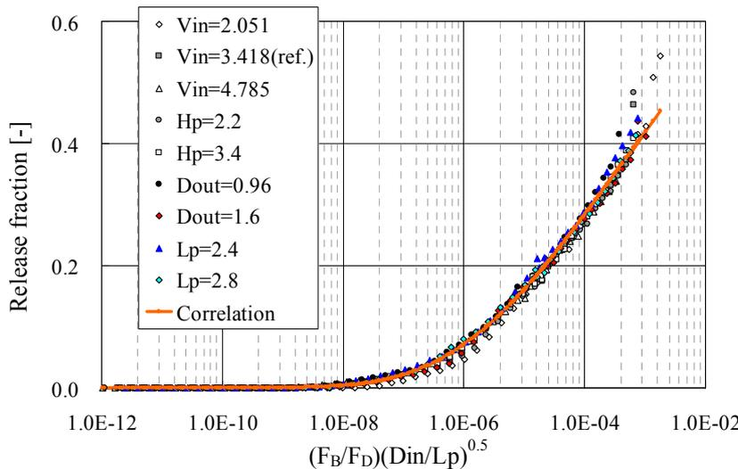
**Fig. 4 Non-Dimensional Expression of Released Bubble Fraction at Free Surface.**
