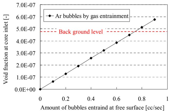
**Fig. 15 Void fraction at the core inlet as a function of the entrained bubble radius (entrained bubble radius is  $1 \mu\text{m}$ )**
