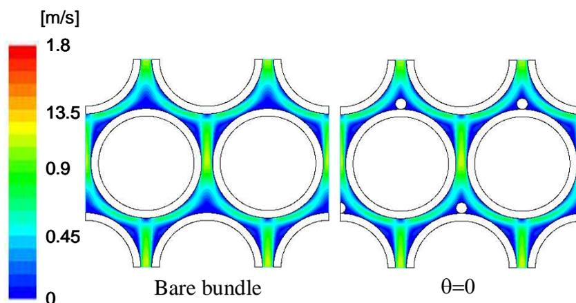
Fig. 8 Comparison of velocity distribution (Bare bundle and 0 degree)
