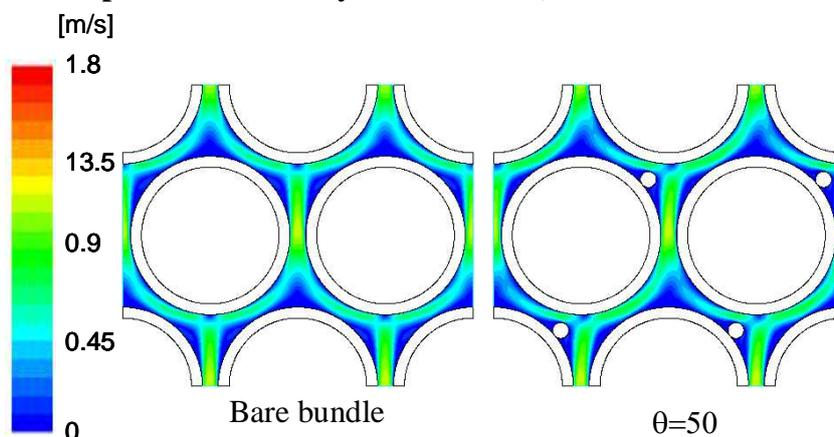
Fig. 9 Comparison of velocity distribution (Bare bundle and 50 degree)
