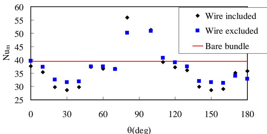
Fig. 7 Nusselt number for each angle of wire attachment
