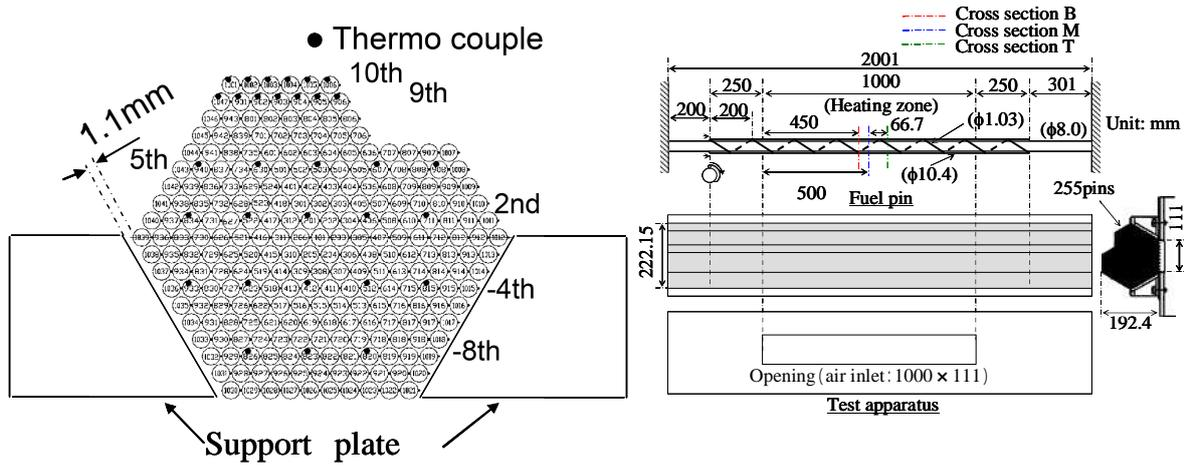
(a) Cross sectional view of apparatus (b) Geometry of apparatus
