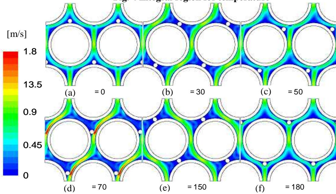
**Fig. 5 Velocity distribution for each angle of wire attachment**
