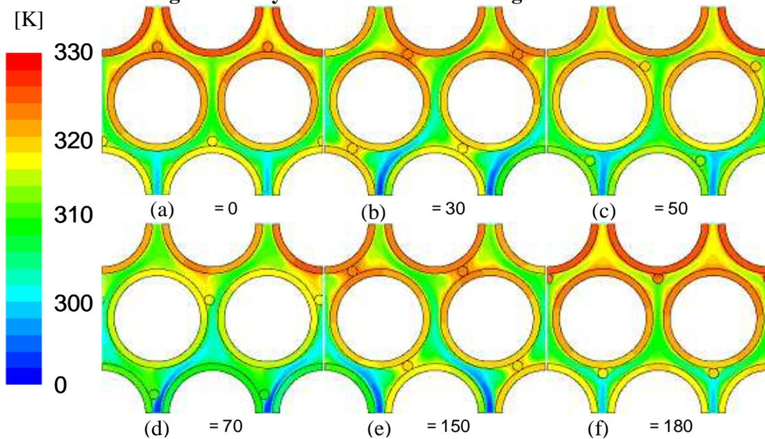
**Fig. 6 Temperature distribution for some angle of wire attachment**
