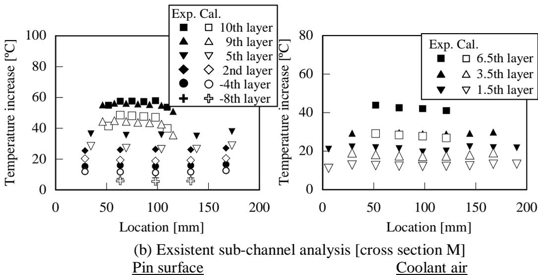
**Fig. 12 Pin surface and coolant air temperature**
