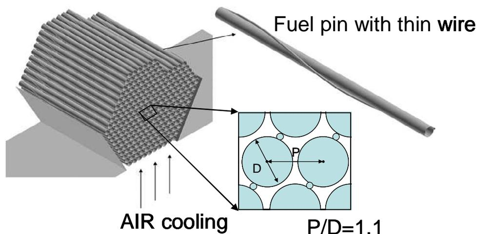
**Fig. 1 Schematic of fabrication process of TRU fuel pin bundle**
