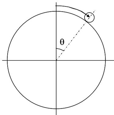
**Fig. 3 Definition of an angle of wire attachment**
