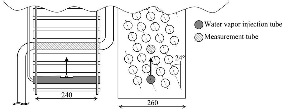
**Fig. 1 Test section of SWAT-1R.**
