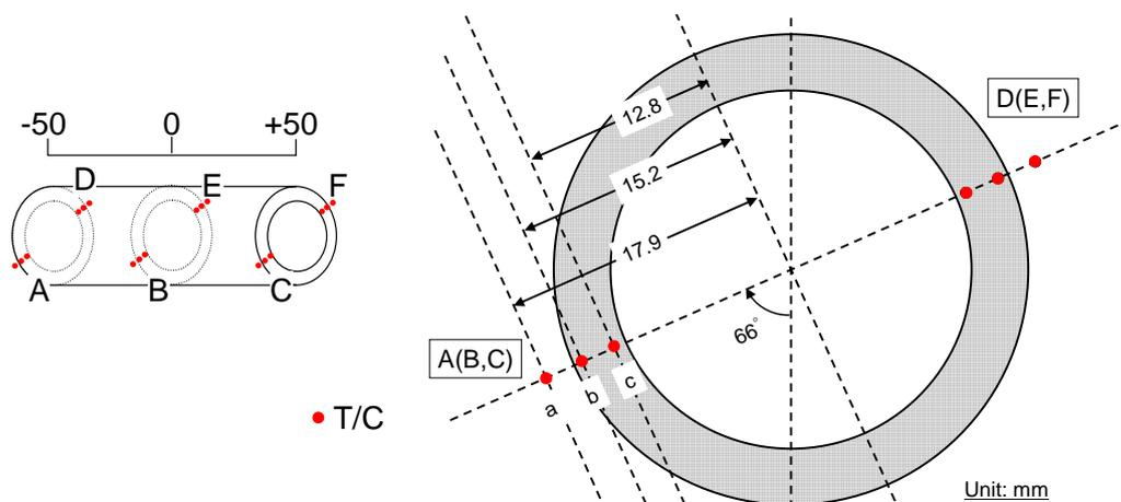
**Fig. 2 Locations and Positions of measurement.**
