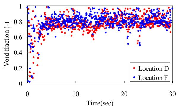
Fig. 8 Transient of Void fraction (top side)
