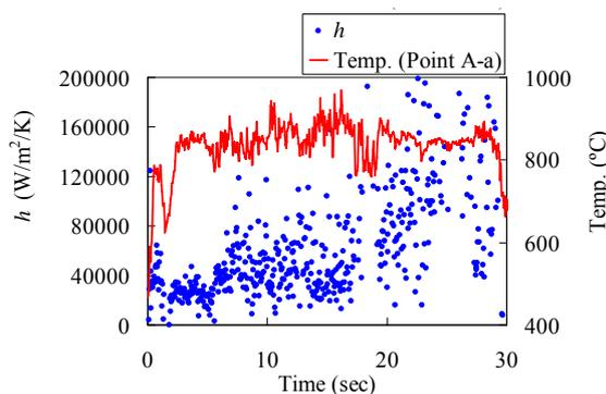
Fig. 3 Heat transfer coefficient at Location A
