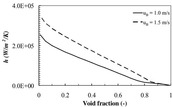
Fig. 5 Correlation diagram of heat transfer coefficient and void fraction
