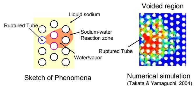
Fig. 1 Sketch of the sodium water reaction phases.
