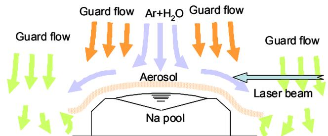
Fig.3 Sodium-water counter flow diffusion flame experiment
