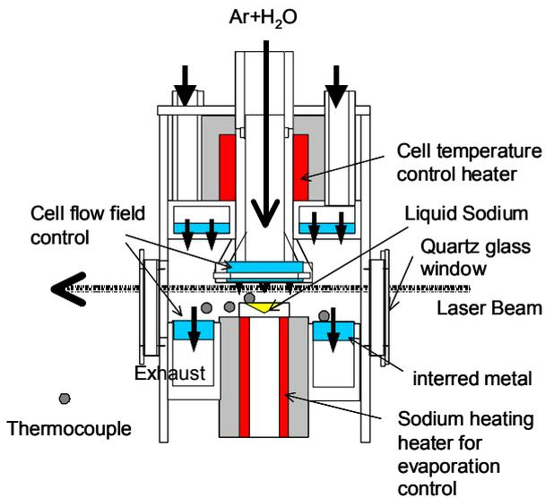
Fig.2 Sodium-water counter flow diffusion flame experiment
