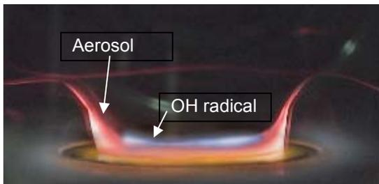
Fig. 5 Visualization of sodium-water reaction (Yamaguchi and Takata, 2006)
