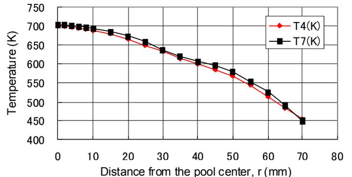
Fig. 7 Radial gas temperature distribution 19mm above the pool surface.
