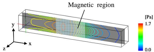
**Fig. 11 Pressure contour ( $\Delta p=0.1$ )**
