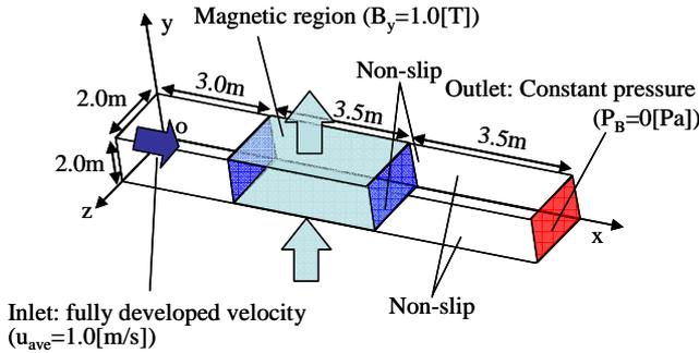
**Fig. 9 Analytical region of rectangular channel flow**
