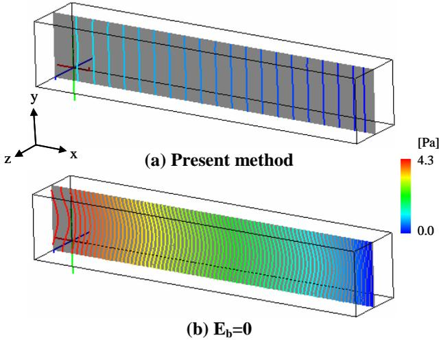
**Fig. 8 Comparison of iso-pressure contours ( $\Delta p=0.05$ )**
