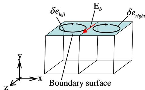
**Fig. 3** Method for giving corrector of boundary electric field
