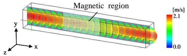
**Fig. 10 Velocity vectors of rectangular channel flow**
