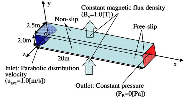
Fig. 5 Hartmann flow analytical region
