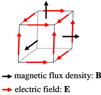
**Fig. 1** Arrangement of **E** and **B** in VFVM
