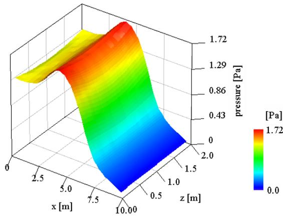
Fig. 12 Pressure change in x-z plane at y=1.0[m]
