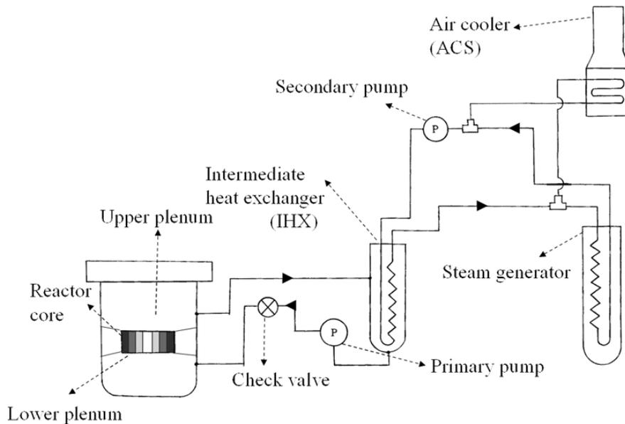
**Fig. 3: Schematic of loop type sodium cooled fast reactor**
