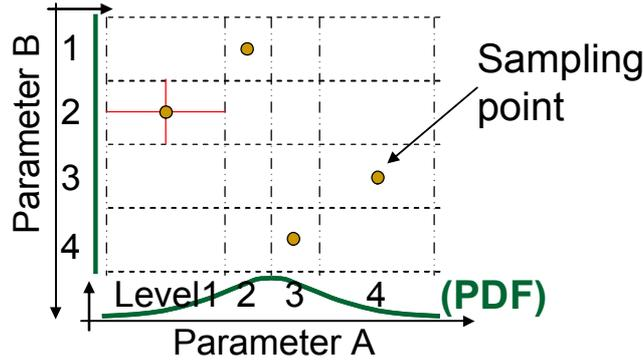
Fig.2: Schematic of LHS
