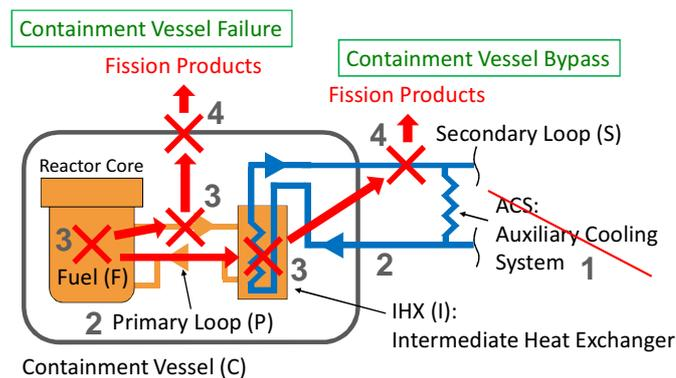
**Fig. 1 LMFBR plant in different accident scenarios**
