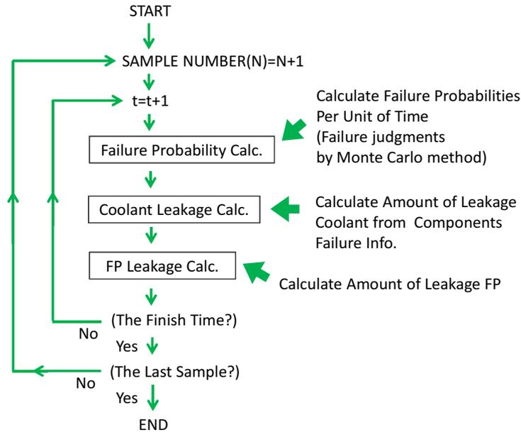
**Fig. 6 Meta-model algorithm**
