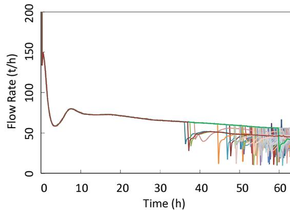
**Fig. 4 Primary-loop flow rate in PLOHS accident analysis (100 samples)**
