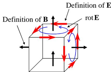
Figure 2 Staggered layout in control volume
