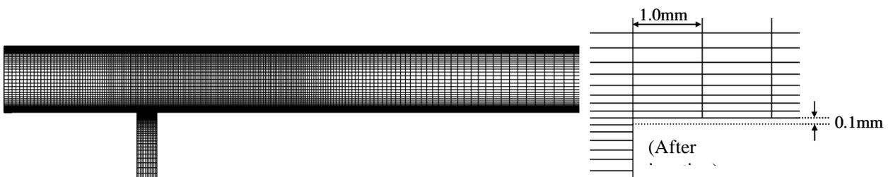
Figure 5 Mesh arrangement
