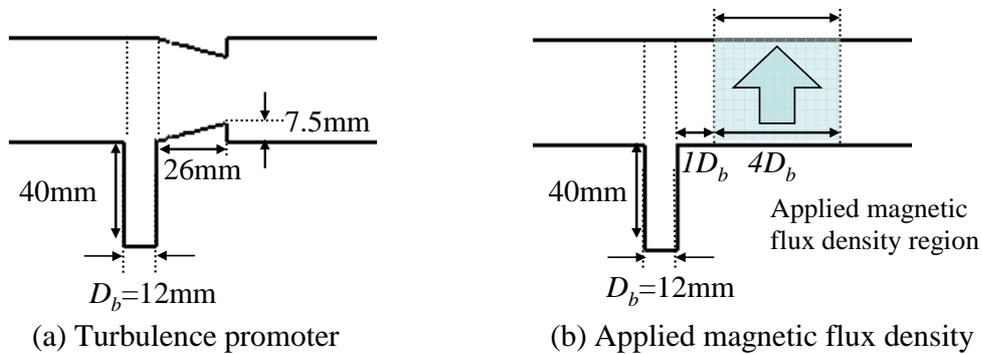
Figure 6 Additional installations for temperature mixing mitigation
