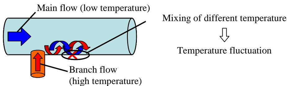
Figure 1 Schematic of temperature mixing after T-junction
