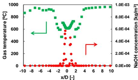
Gas temperature and NaOH concentration on tube surface
