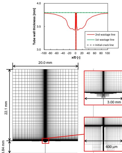
**Fig. 15** The shape of the tube surface and the second remeshing model for SHDP
