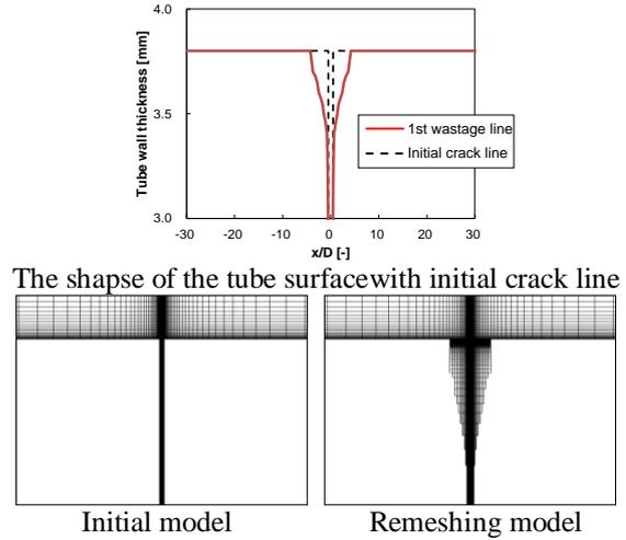
Fig. 3 Construction of wastage remeshing model
