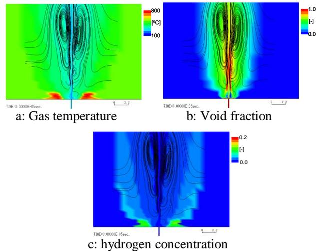
Fig. 6 Results of the initial model at  $3.0\times 10^{-5}\text{s}$
