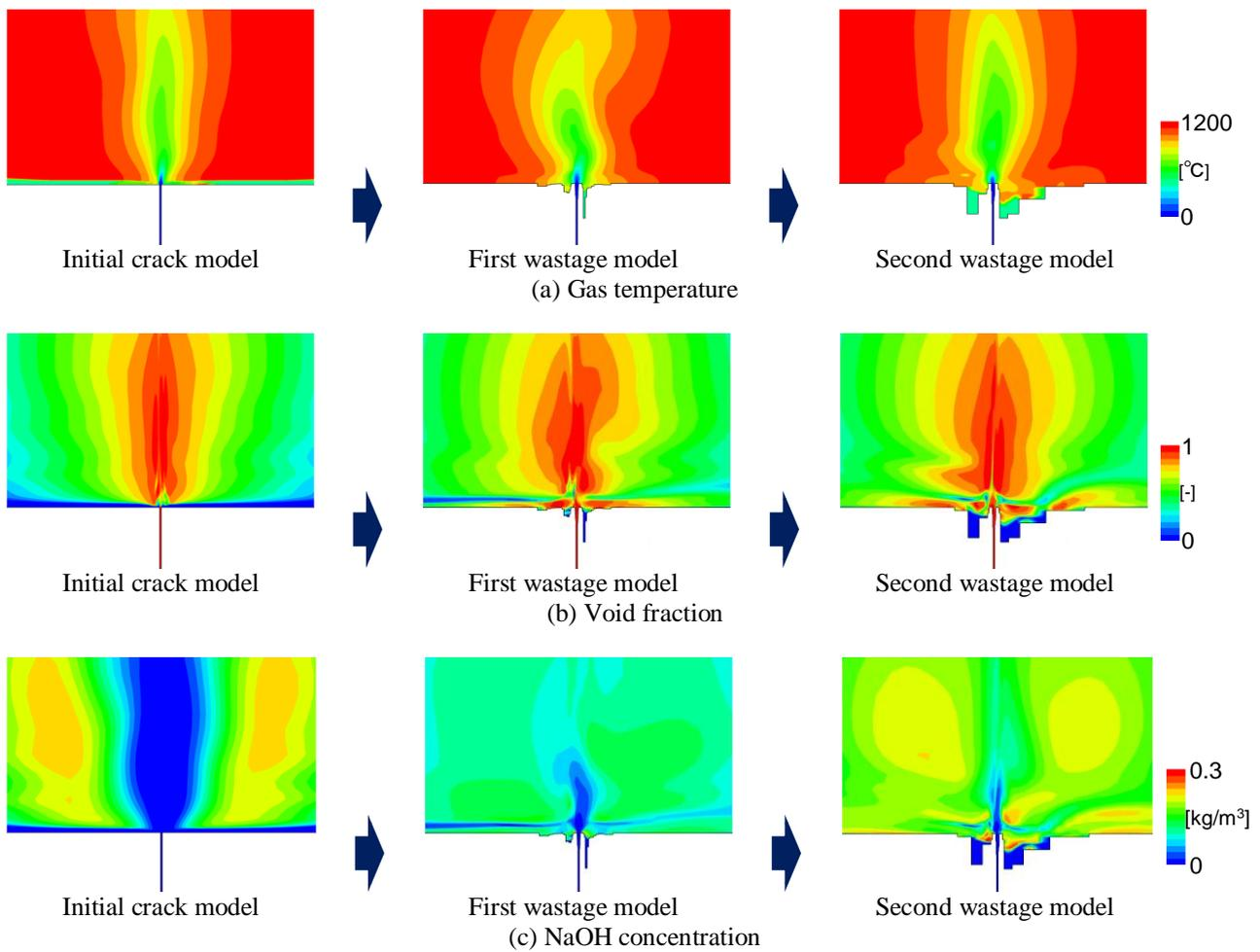
**Fig. 18 Results of the crack enlargement model (GTDP)**
