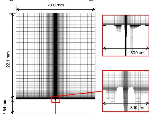
**Fig. 12** The first wastage remeshing model for GTDP
