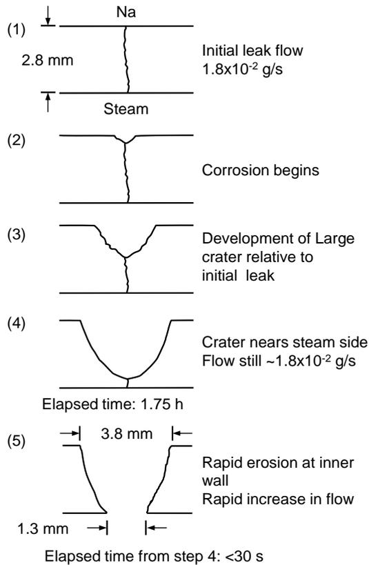
**Fig. 1 Process of crack enlargement by self-wastage**
