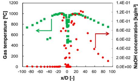
**Fig. 14** Result of the first wastage model under SHDP at  $8.0 \times 10^{-4}$  s
