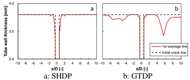
**Fig. 10** The shapes of the tube surface after first self-wastage analysis
