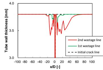
**Fig. 16** The shape of the tube surface and the second remeshing model for GTDP
