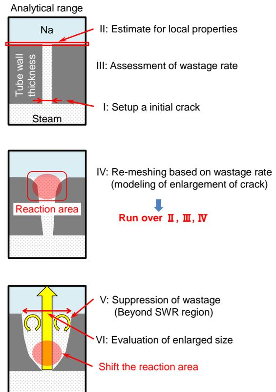
**Fig. 2 Numerical procedure for the self-wastage analysis**
