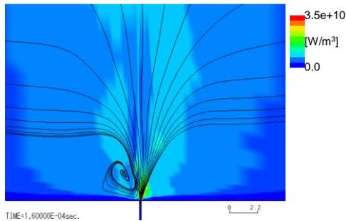
**Fig. 8** Heat generation of a surface reaction at  $1.6 \times 10^{-4}$ s
