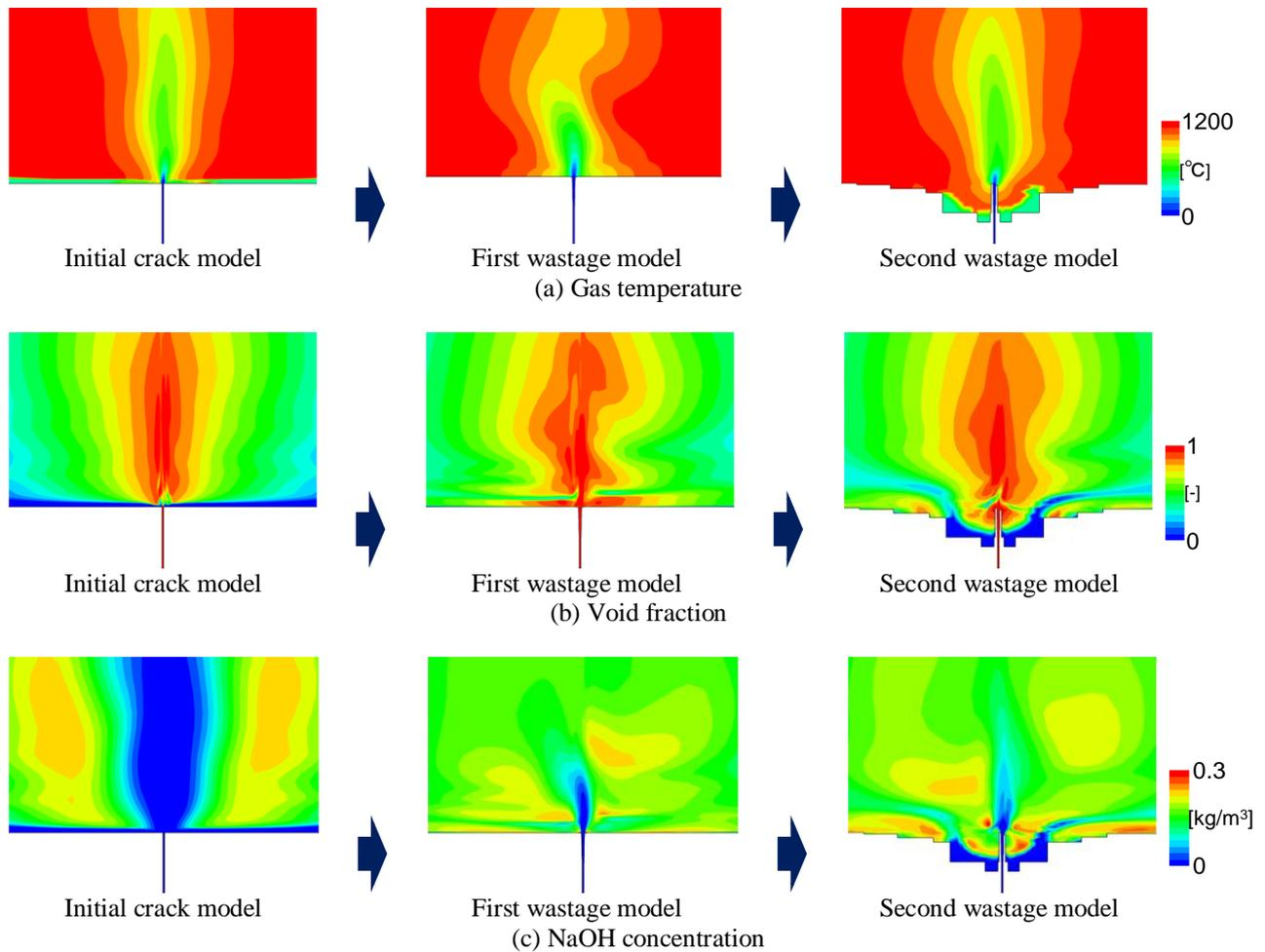
**Fig. 17 Results of the crack enlargement model (SHDP)**
