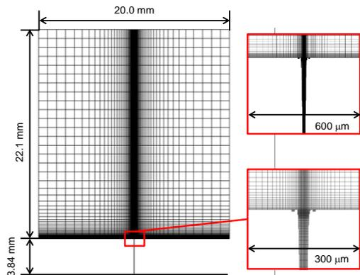
**Fig. 11** The first remeshing model for SHDP
