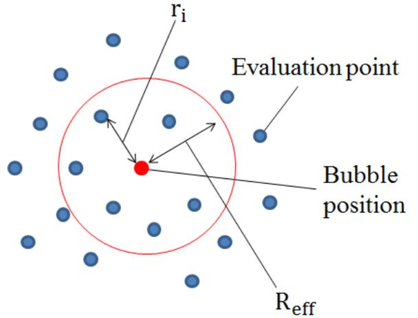
**Fig. 1 Interpolation between bubble and flow field**
