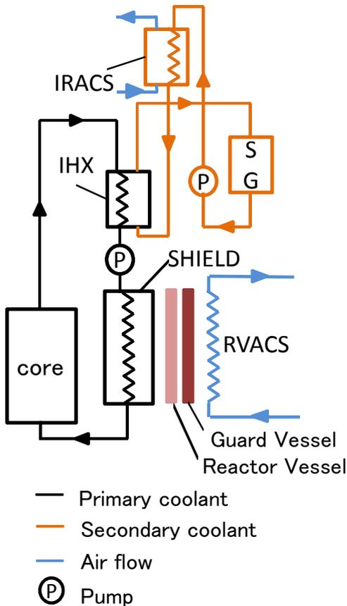
Fig.4 Model flow of 4S reactor
