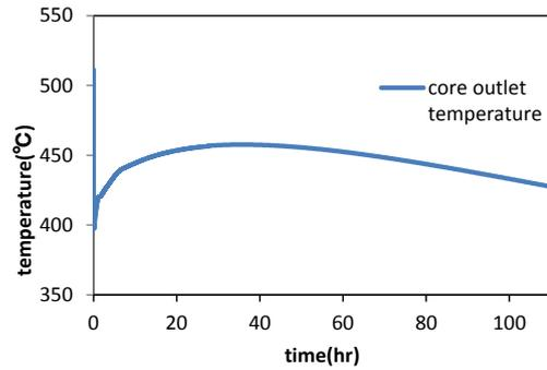
Fig.5 Typical transient coolant temperature (Core outlet)
