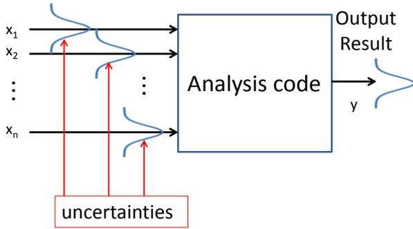
Fig.1 Conceptual diagram of BEPU analysis
