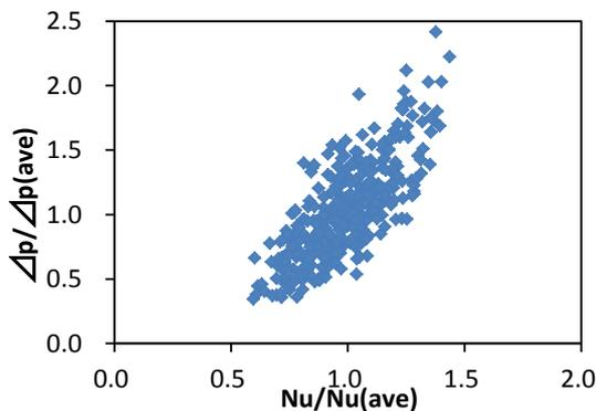
**Fig.8 Variance of pressure drop and heat transfer coefficient in each sample (BEPU based on scaling laws)**
