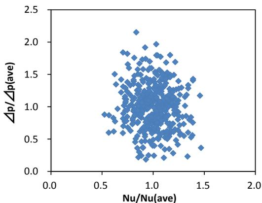
**Fig.9 Variance of pressure drop and heat transfer coefficient in each sample (normal BEPU)**
