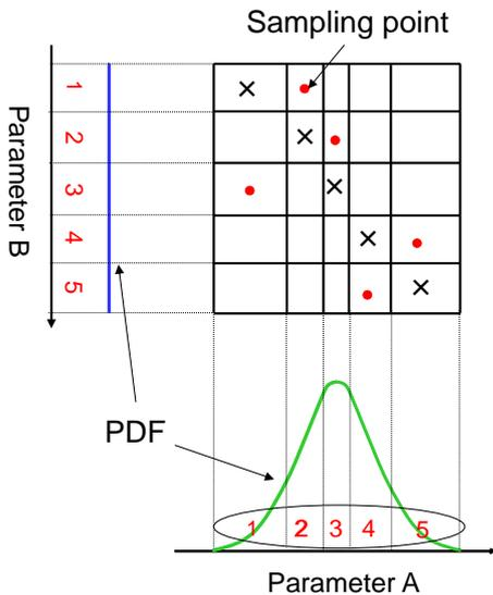
Fig.2 Schematic of LHS
