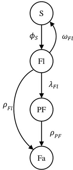
**Fig. 3 Markov model for degradation of defense barrier**
