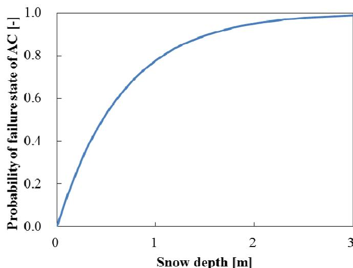
**Fig. 4 Probability of Failure State of AC.**
