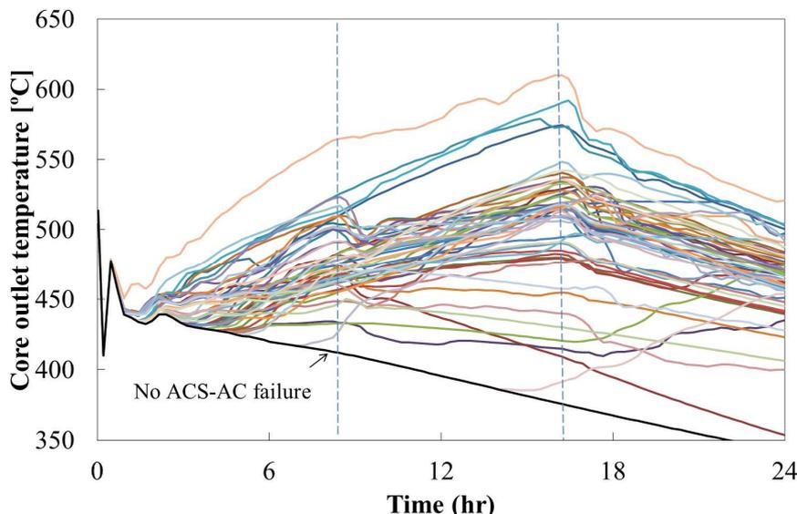
**Fig. 6 Time Transient of Core Outlet Temperature with Snow Removal.**
