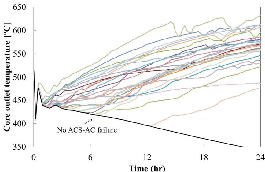
**Fig. 5 Time Transient of Core Outlet Temperature in case of No Snow Removal.**
