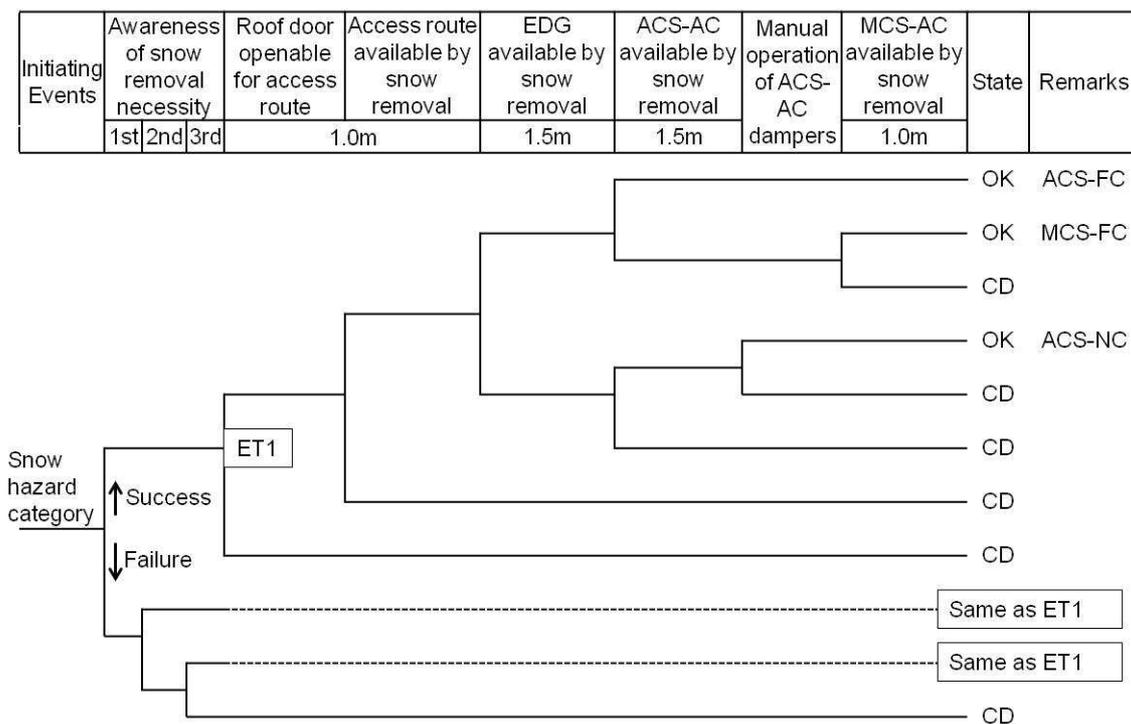
NB) CD: Core Damage, EDG: Emergency Diesel Generator, ACS: Auxiliary Cooling System, MCS: Maintenance Cooling System, AC: Air Cooler, FC: Forced Circulation, NC: Natural Circulation
