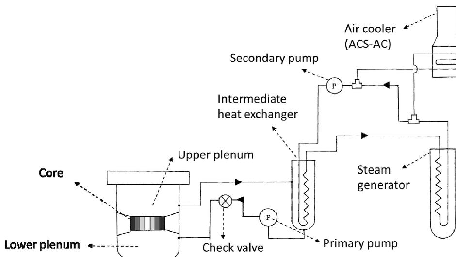
**Fig. 3 Schematic of Heat Transport System in SFR.**
