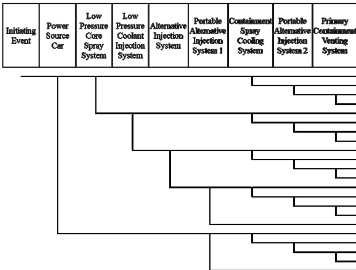
**Fig.6 ET for Containment Failure**
