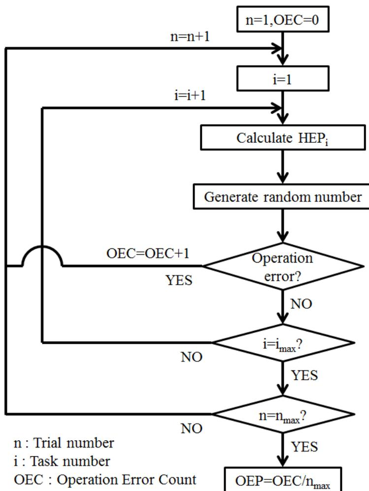
Fig. 4 Flowchart of Monte Carlo simulation.
