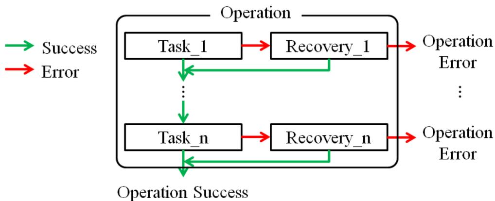
**Fig. 1 Example of operation in THERP.**
