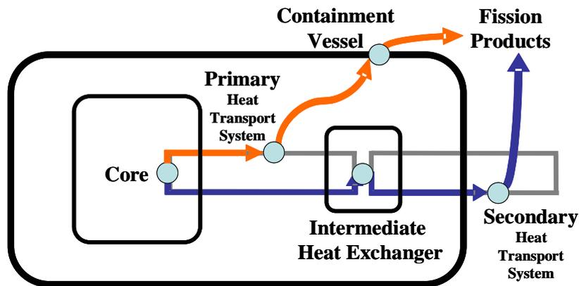
Figure 4: Leakage paths of the Fission Products
