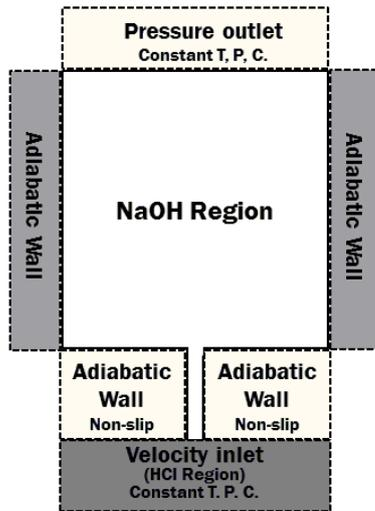
Figure 3. Boundary conditions for the domain
