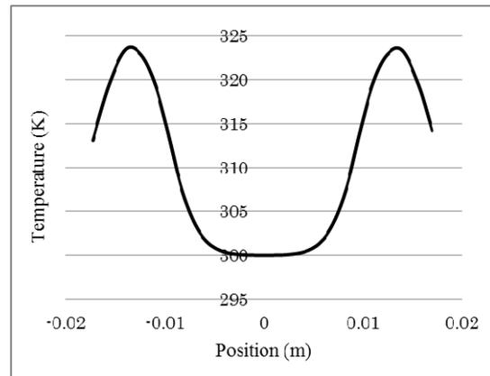
Figure 5. Temperature distribution at the nozzle surface (at  $Y=1.0E-2 [m]$ )
