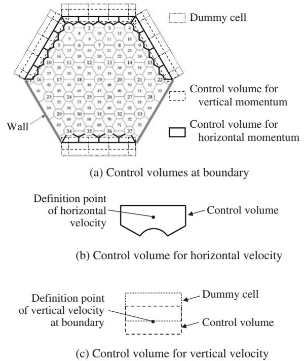
**Fig. 3** Additional control volume for boundary condition
