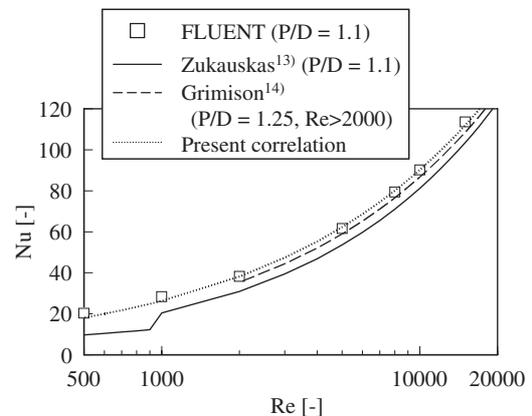
**Fig. 6** Comparison of heat transfer correlations
