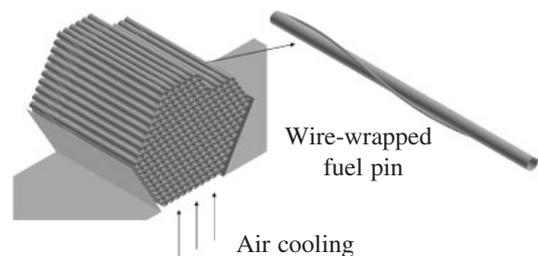
Fig. 1 Schematic image of TRU fuel bundle and its cooling
