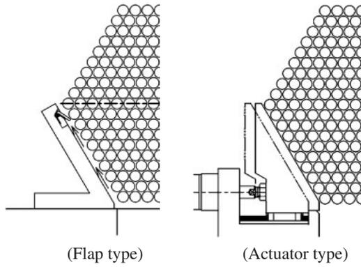
Fig. 10 Mechanical image of clearance arrangement
