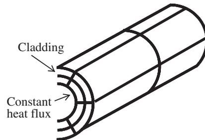
**Fig. 4** Nodalization of cladding
