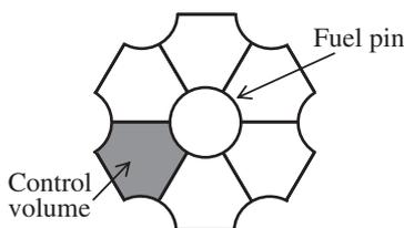
**Fig. 2** Specified control volume in subchannel analysis
