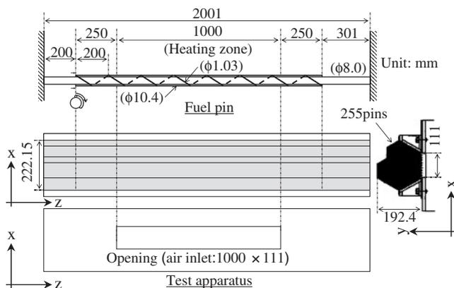
**Fig. 7** Full mock-up pin bundle test apparatus
