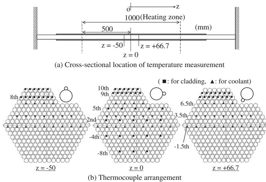
Fig. 9 Location of temperature measurement in experiment
