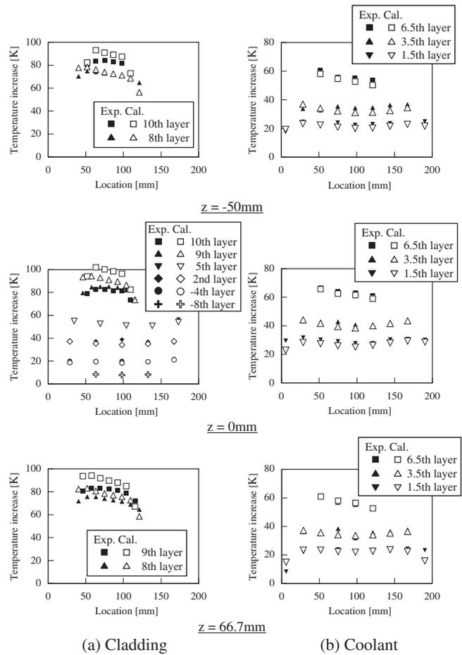
Fig. 12 Comparison of cladding and coolant temperatures (Clearance: 5 mm, without natural convection)
