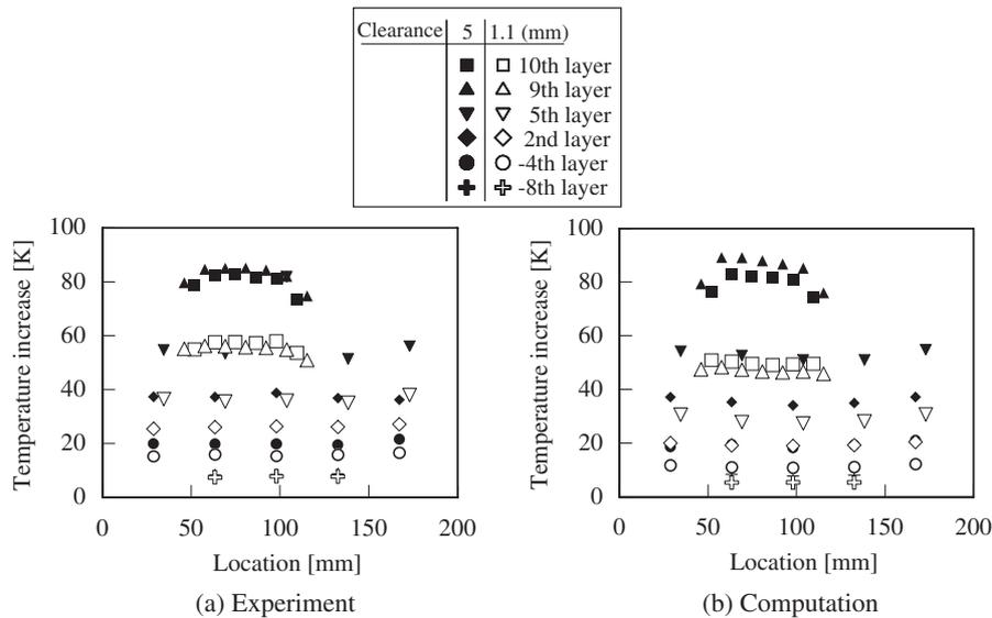
Fig. 18 Influence of clearance on cladding temperature at  $z = 0$  mm
