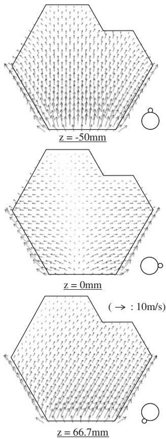
**Fig. 13** Velocity distribution at  $z = 0\text{ mm}$  (Clearance: 5 mm, without natural convection)
