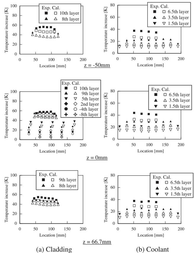
**Fig. 17** Comparison of cladding and coolant temperatures (Clearance: 1.1 mm, with natural convection)
