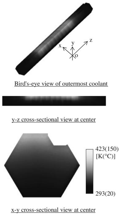
**Fig. 16** Coolant temperature distribution of benchmark analysis (Clearance: 1.1 mm, with natural convection)
