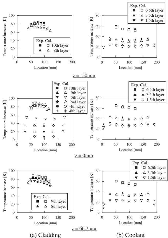
**Fig. 15** Comparison of cladding and coolant temperatures (Clearance: 5 mm, with natural convection)
