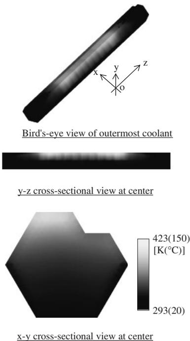
Fig. 11 Coolant temperature distribution of benchmark analysis (Clearance: 5 mm, without natural convection)
