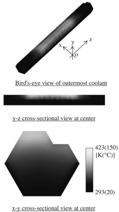
**Fig. 14** Coolant temperature distribution of benchmark analysis (Clearance: 5 mm, with natural convection)
