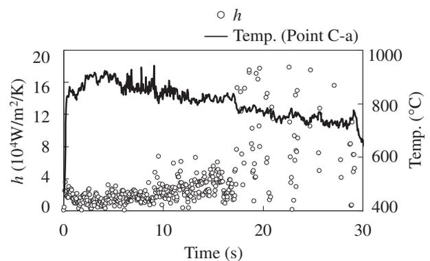
**Fig. 9** Heat transfer coefficient at Location C
