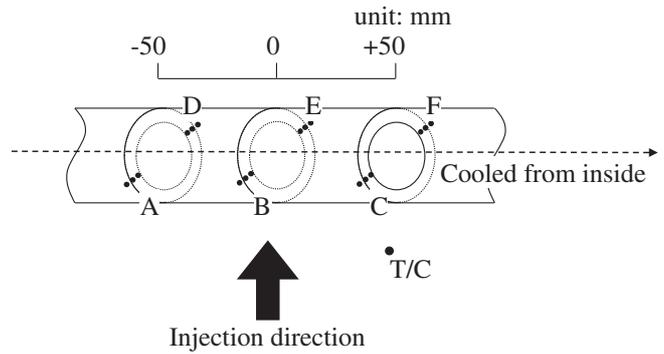
Fig. 3 Measurement tube
