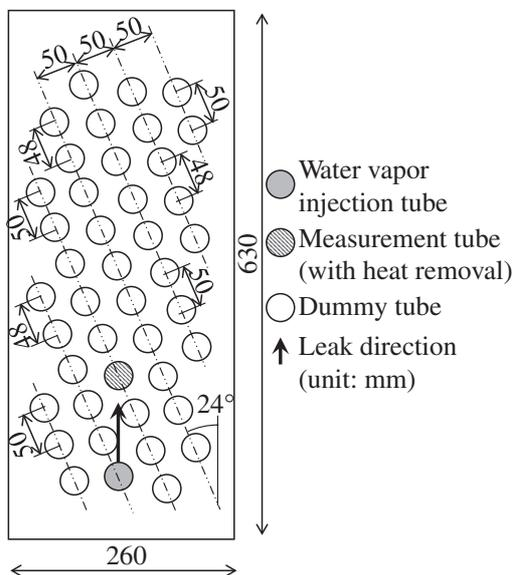
Fig. 2 Test section of SWAT-1R
