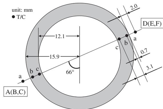
Fig. 4 Position of T/C
