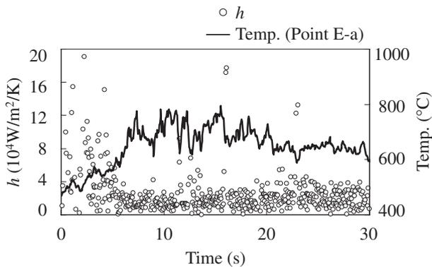
Fig. 11 Heat transfer coefficient at Location E
