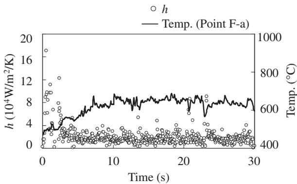
Fig. 12 Heat transfer coefficient at Location F
