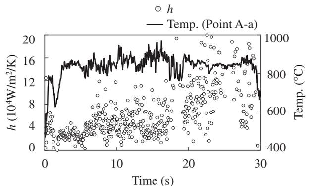
Fig. 6 Heat transfer coefficient at Location A
