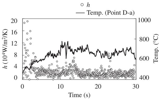
Fig. 10 Heat transfer coefficient at Location D
