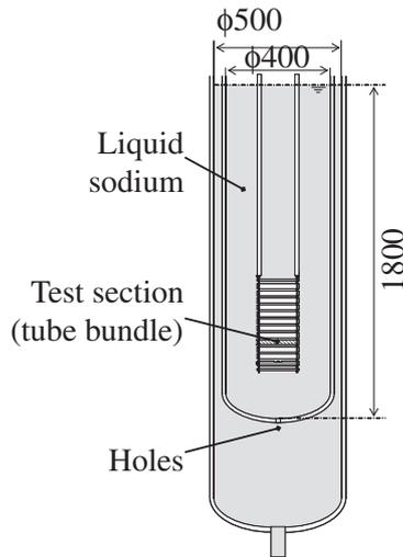
Fig. 1 SWAT-1R test vessel
