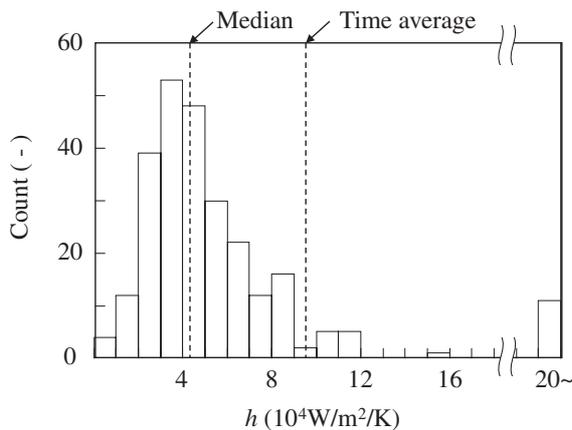
**Fig. 7** Histogram of HTC during 5–18 s at Location A
