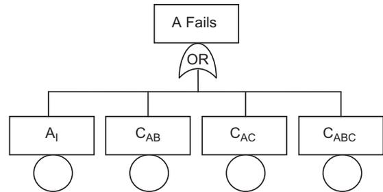
Fig. 2. Expanded CCBE fault tree for component A.
